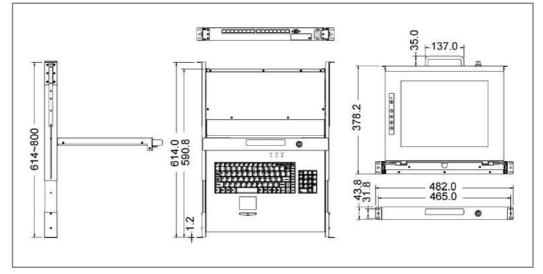
Figure 1-2. 15" LCD console with 16-port CAT5 KVM Dimension
