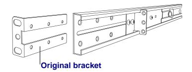
2 Input rear long bracket to rear of the rail then adjust rear bracket to fit your cabinet. Tight-up 2~3 screws upon the length you need. One is forbidden.
