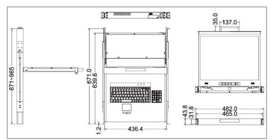
Figure 1-10. 20" LCD console with 8-port CAT5 KVM Dimension
