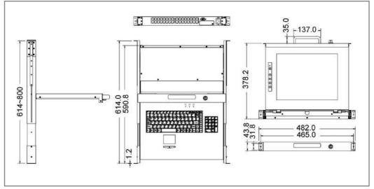
Figure 1-3. 15" LCD console with 32-port CAT5 KVM Dimension
