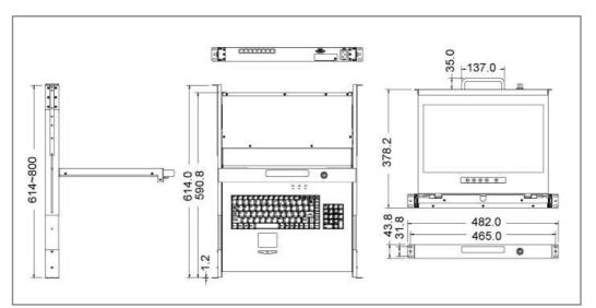
Figure 1-4. 17" Full HD LCD console with 8-port CAT5 KVM Dimension
