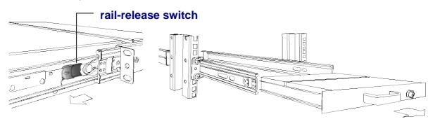
6. Push rail-lock switch on the rail and push rail back.(Both sides)
