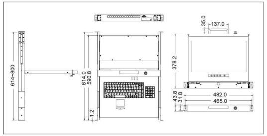
Figure 1-5. 17" Full HD LCD console with 16-port CAT5 KVM Dimension
