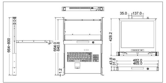
Figure 1-8. 19" LCD console with 16-port CAT5 KVM Dimension
