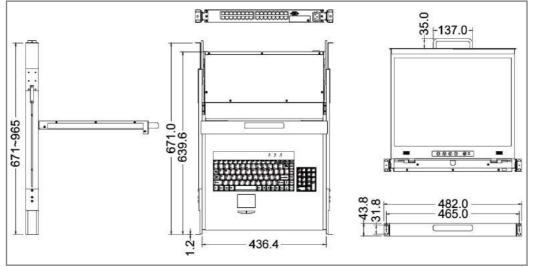
Figure 1-12. 20" LCD console with 32-port CAT5 KVM Dimension
