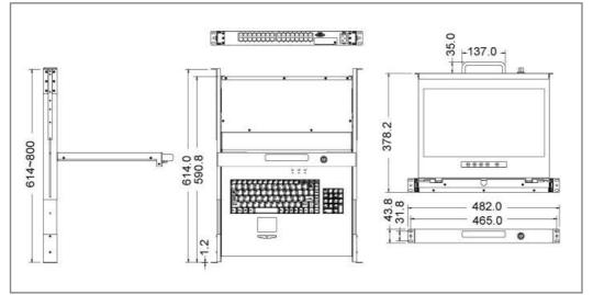
Figure 1-6. 17" Full HD LCD console with 32-port CAT5 KVM Dimension
