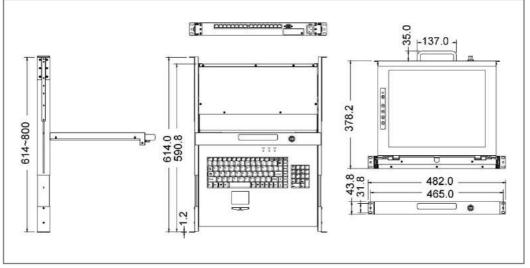
Figure 1-5. 17" LCD console with 16-port CAT5 KVM Dimension
