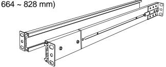
2. Long bracket x 2. (Needed for rack depth 828 ~ 1000mm)
