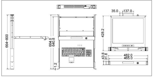
Figure 1-9. 19" LCD console with 32-port CAT5 KVM Dimension
