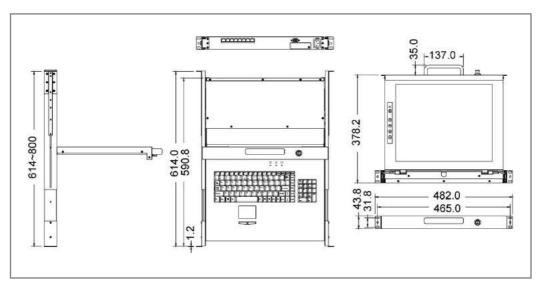
Figure 1-4. 17" LCD console with 8-port CAT5 KVM Dimension
