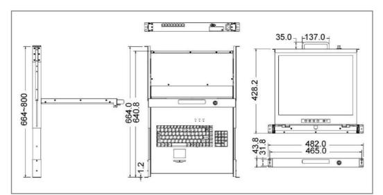
Figure 1-7. 19" LCD console with 8-port CAT5 KVM Dimension
