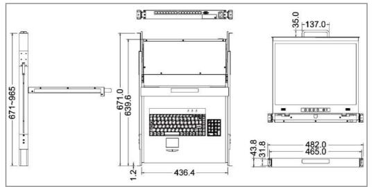
Figure 1-11. 20" LCD console with 16-port CAT5 KVM Dimension
