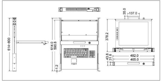
Figure 1-6. 17" LCD console with 32-port CAT5 KVM Dimension
